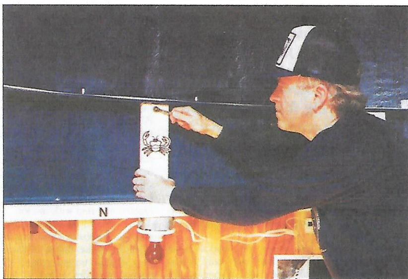
At the suggestion of his friend Bob Custer, Castle (pictured) modified the support system of his dome. He used longer bolts than originally supplied on the axles of the roller wheels and placed wooden braces on the inside ends of the bolts. Although early versions of the dome had 12 rollers, current units are equipped with 16.
