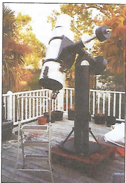
Left: Phillips's observatory was built around his telescope and pier, which are permanently installed on a small deck over his kitchen. Limited space had ruled out earlier designs that called for a roll-off roof or lifting a dome with a crane. All photographs with this article are by the respective authors. Right: Jim Phillips with his 10-foot Home-Dome. The observatory was built and the dome assembled by two carpenters who had no previous experience working on an observatory.
