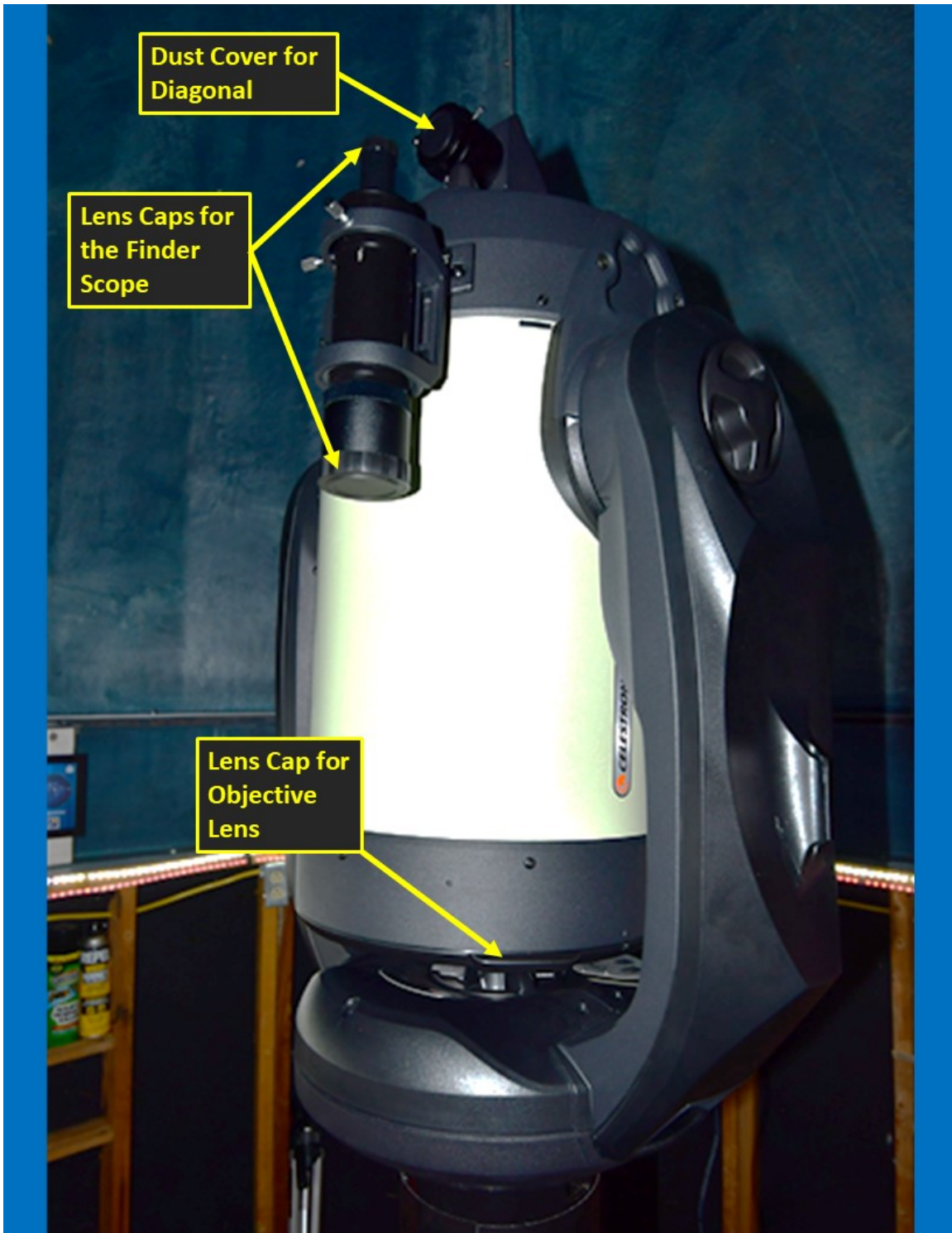
Figure 12: Before placing the cloth cover over the telescope (before leaving the observatory), install the telescope's objective lens cap, the lens caps for both ends of the finder scope and the dust cover for the eyepiece diagonal. Then position the telescope pointed down as shown here. Note: The Lens Cap for the Objective must be rotated to engage and lock it to the front of the telescope.
