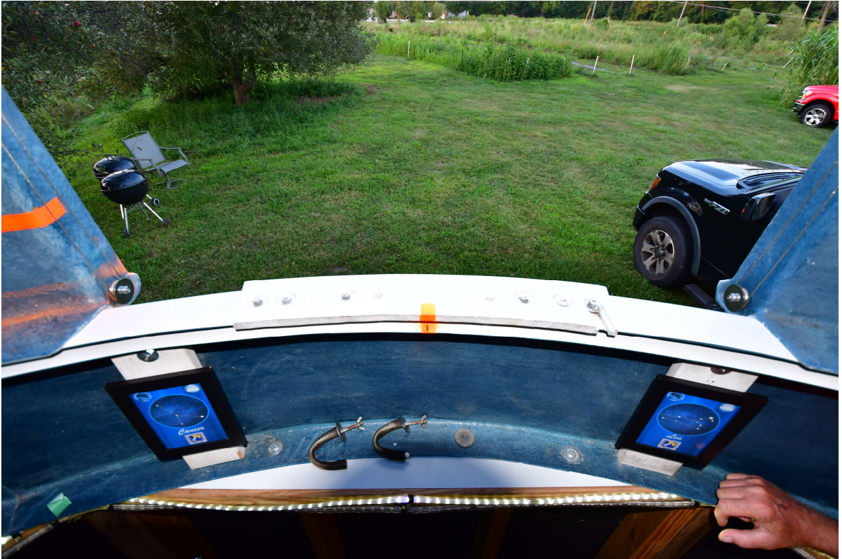
Figure 9: Before closing and clamping down the shutter doors, rotate the dome to align the orange colored markings shown. This “home position” marks the correct position for insertion of the J-hook clamps to secure the shutter doors.
