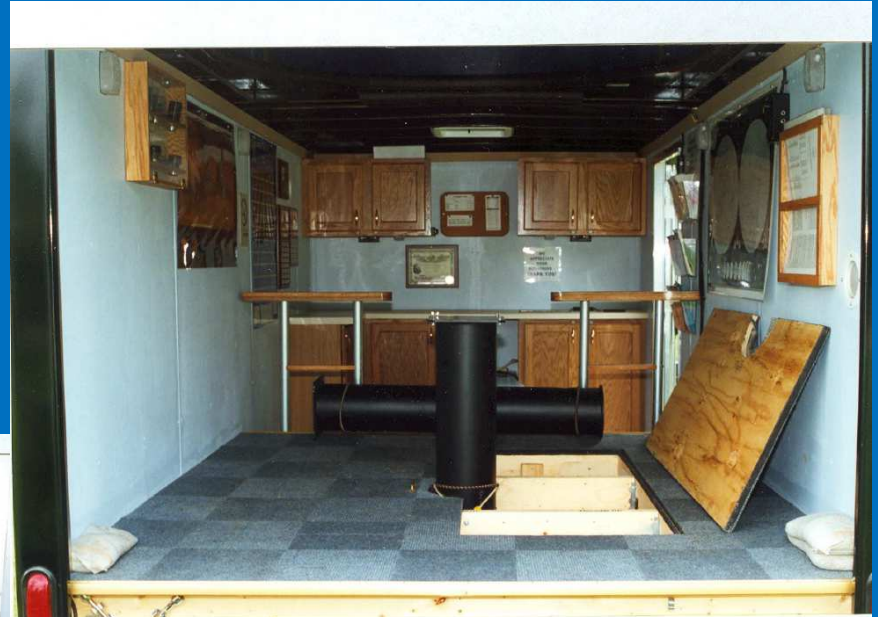
Looking toward the front of the trailer. Pier is in transport mode. One half of the Observing Deck Access Door is shown open.
