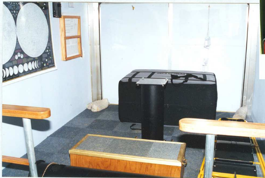
Looking toward rear of trailer when it is ready for transport. Telescope is in the carrying case. Outside step is placed next to upper pier, the ladder is folded and lies flat.
