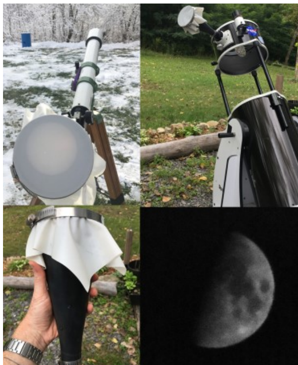
Sun Funnels shown in action: Starting clockwise from the bottom left, a standalone Sun Funnel; attached to a small refractor to observe the transit of Mercury in 2019; attached to a large telescope in preparation for evening lunar observing; projection of the Moon onto a funnel from a medium-size scope (5 inches) .
