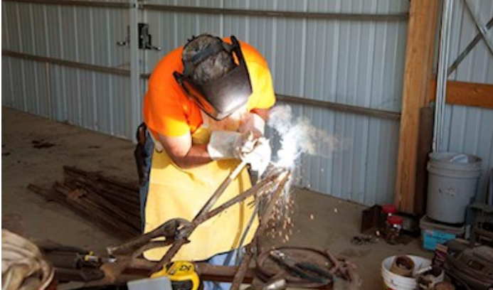
Rusty constructing the rebar structure (the day before) to be inserted into the tube for strengthening and support
