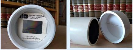
Home-made spectroscope, 500-lines-mm film, 12.5° bend SA 100 Grating Filters can also be used
