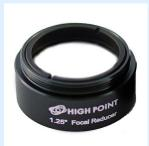
**Field Flattener with Focal Reducer**. Often used to make the full image sharp (and flat) without star elongations on the sides. They include a 0.8x **Focal Reducer - to reduce an f-7 focal ratio to f-5.6**. Note: An M42 x .75" extension tube or spacer ring may be needed to make sure the back focus (distance from the back of the flattener to the sensor) matches that of the flattener/reducer (55 mm). Note: A 0.8x Focal Reducer also divides the magnification of the eyepiece.
